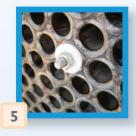
Plug is securely fastened when torque wrench clicks once.
