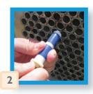
You may need to tighten plug slightly before installing to get a snug fit. Alternatively, you may need to loosen nut and stretch silicone to fit.
