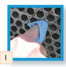
Make sure the tube is free of excess debris at the opening. (wipe with rag if necessary)
